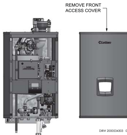
Figure 1 Remove upper and lower front access panels
